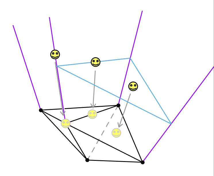
We still need to handle the positions that fall outside of the hull of the probes, ideally by smooth extrapolation of the probes that form the hull.
