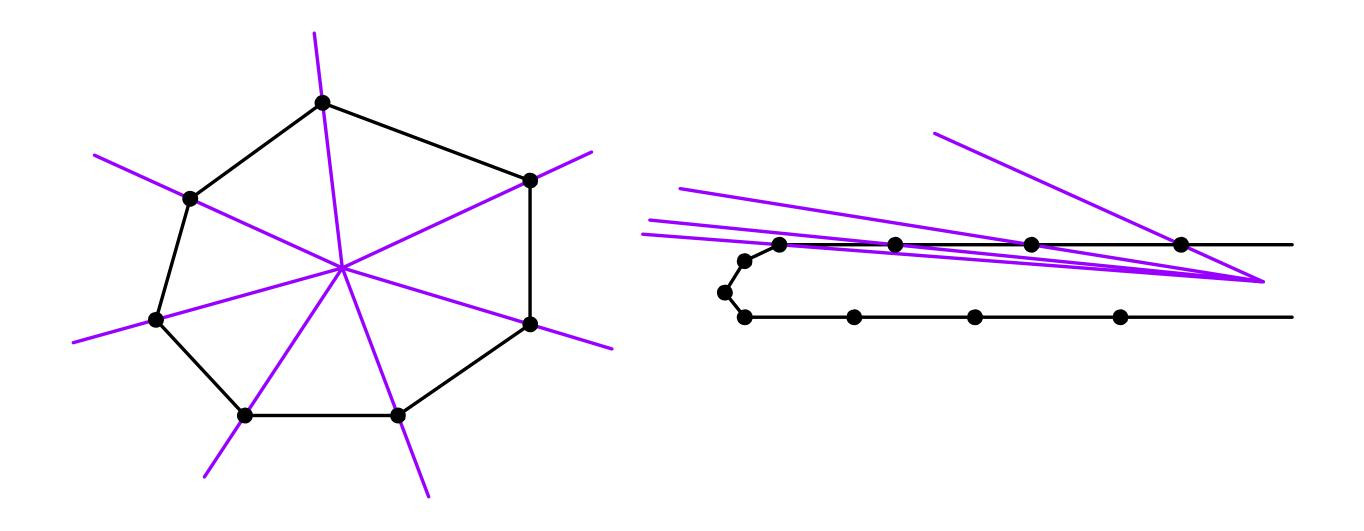
The requirement of all rays intersecting at one position leads to badly-shaped outer cells if the probe set happens to be not very round.
