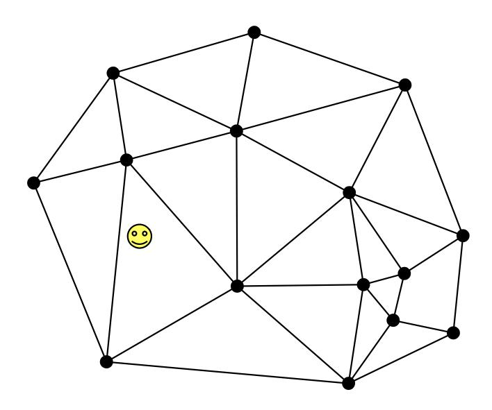
Let's triangulate that set. Delaunay triangulation is the optimal triangulation if we can't modify the set of points and want to avoid skinny triangles.
