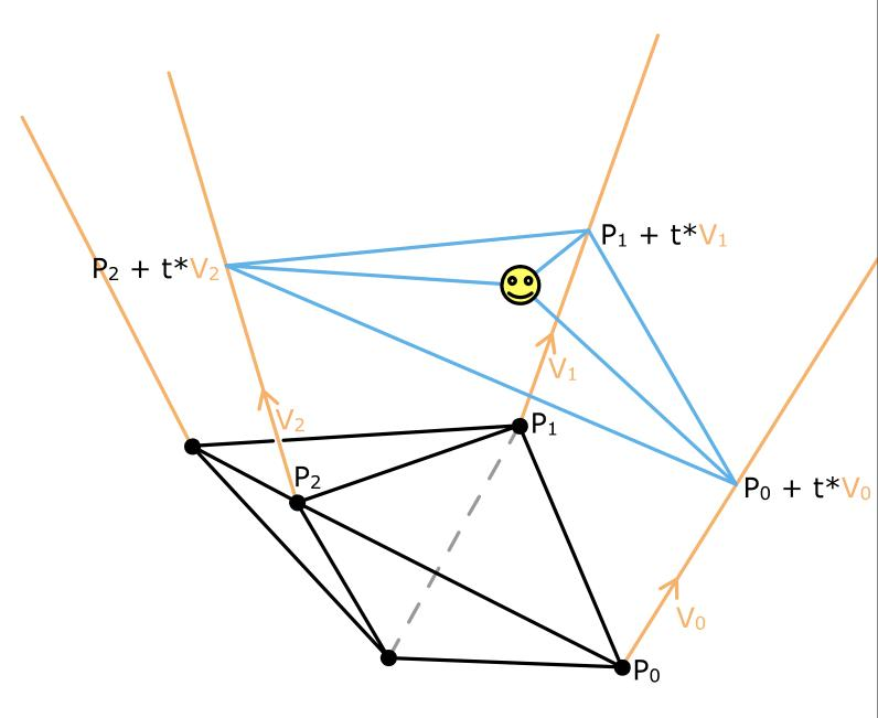
Once we've found t, we can calculate barycentric coordinates of the object within the blue triangle and these are our weights for the 3 probes forming that outer cell.
