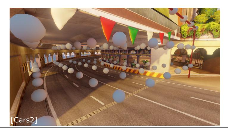
Typically probes are arranged in 3D regular grids to enable trilinear interpolation.
