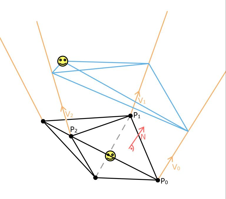
When performing the search, we pretty much proceed as before. The only difference is that we first check if we're still above the hull face by testing the dot with the (red) normal. Outer cells have 4 neighbours, just like tetrahedra.
