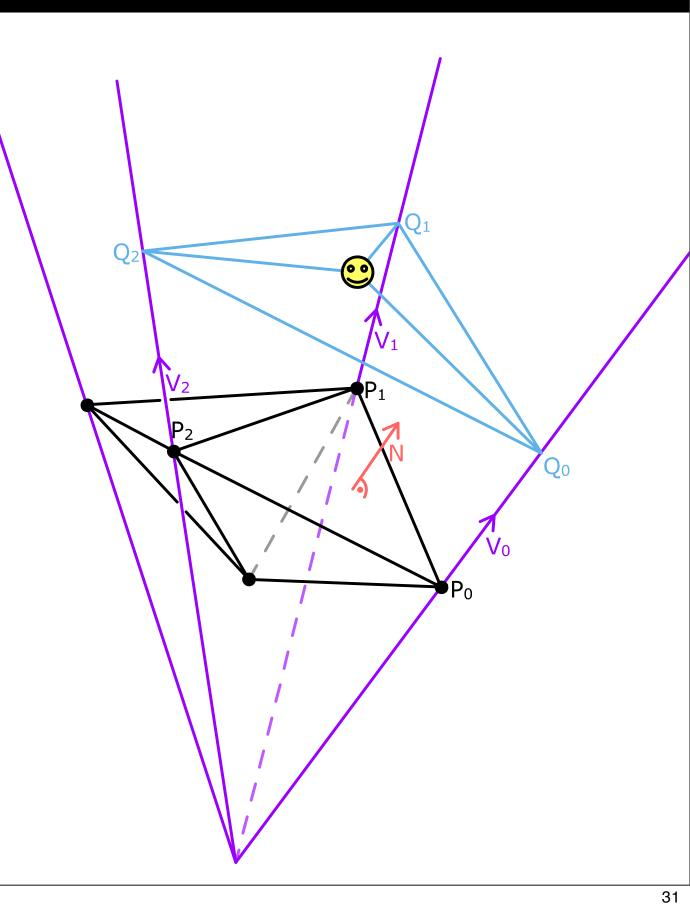
One solution is to form the outer cells by extruding the hull faces along rays, which all meet at the centre of the entire mesh. The math is very easy in that case, but there's a problem.
