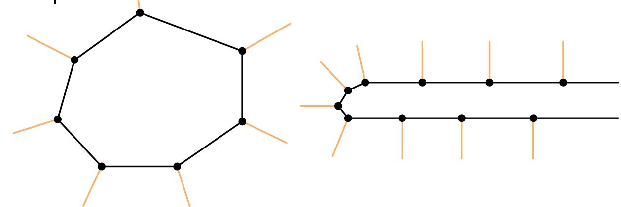
Ideally the outer cells should be roughly perpendicular to the surface. We can do that by spanning the outer cells between the vertex normals. In 3D the problem is that adjacent normals aren't necessarily coplanar, so the resulting shapes will be those twisted or warped prisms, but let's try to deal with that.
