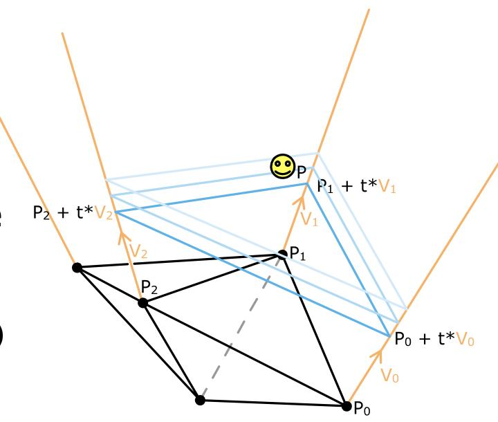
If we look at the image, P0, P1, P2 is an outer face. The rays extending from each of those 3 vertices are forming the outer cell, which extends to infinity. V0, V1, V2 are the direction vectors of those rays. To get any point on the ray 0, we just take P0 + t\*V0, where t goes from 0 to infinity.
