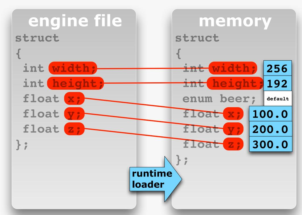
Now that we know how the data in the file is laid out, and the runtime knows how the data needs to be laid out in memory, we can match each data field in memory with one in the data file.
