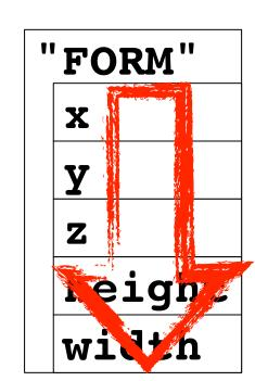
The reader reads through the fields, one by one, and writes the data in the runtime structure, one field at a time.
