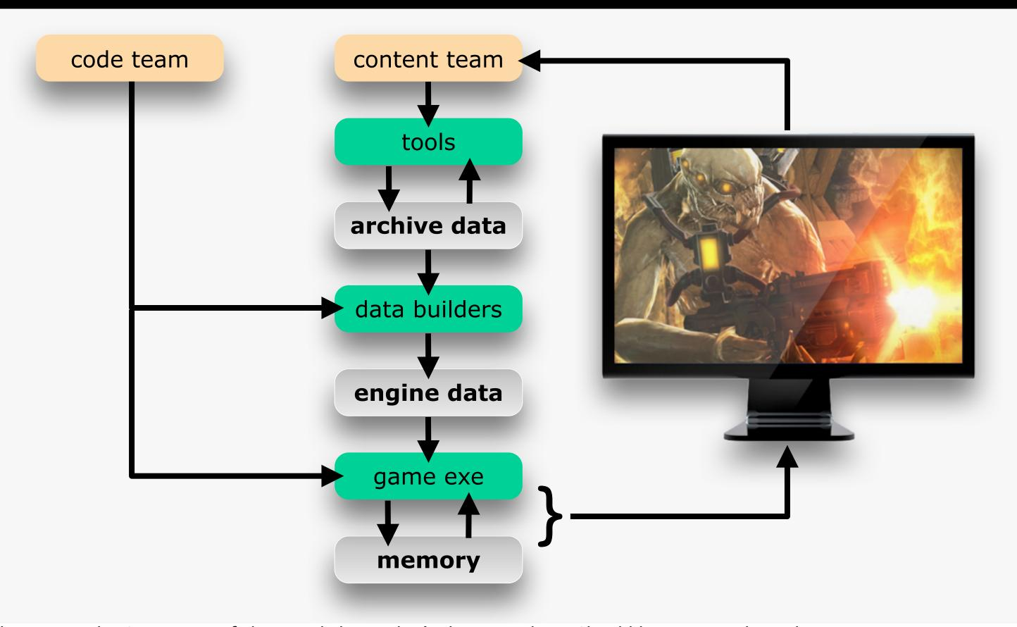
Remember this production pipeline? Assertions fail routinely here. That's the wrong loop! Should be going to the code team.
