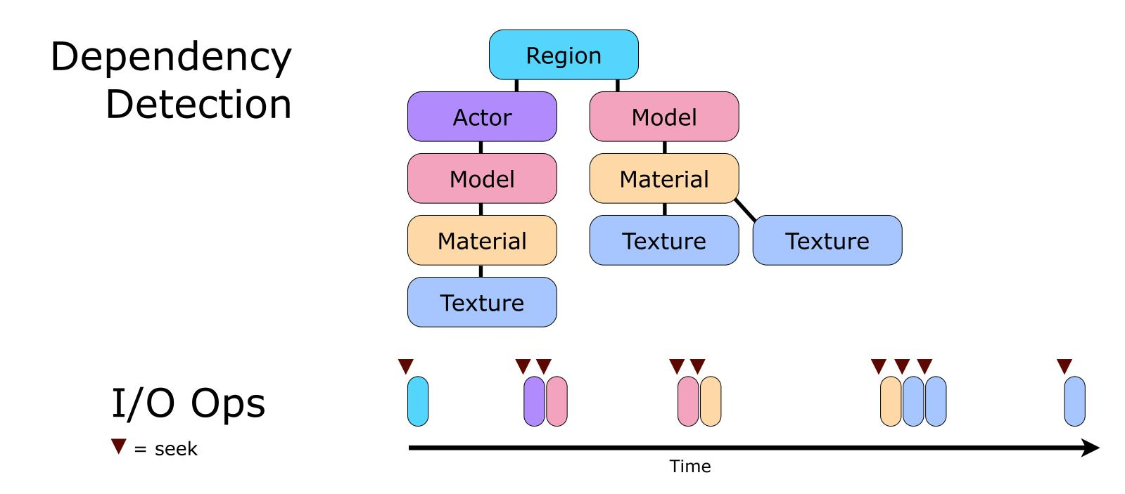
Simplified model of the loose loading scheme. Consider a region with a static model and an actor (visually represented by a model).
