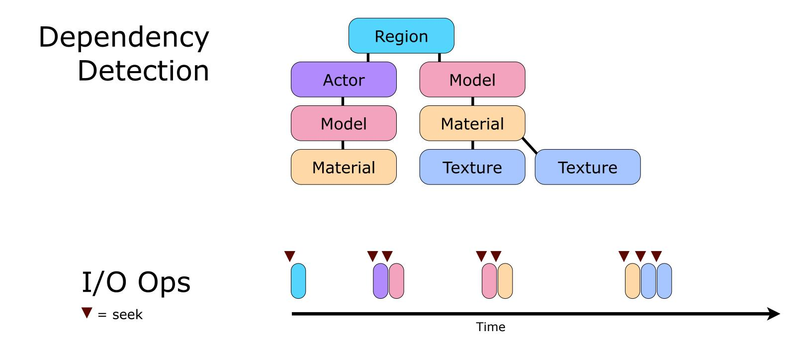
Simplified model of the loose loading scheme. Consider a region with a static model and an actor (visually represented by a model).
