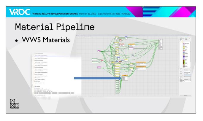
For the new engine we decided that we would have all our shaders go through Materials, which is Sony World Wide Studios shared node based material editor, in part because the backend shader code had become an order of magnitude more complex, making the barrier to entry even higher. In the new engine the lighting code is still handled with hand written code, with surface parameters like albedo, gloss, normals being plugged in to this black box.
