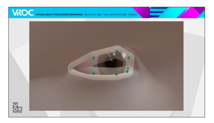
Better still, as the eye is roughly spherical we can project the joint positions onto the eyeball surface reasonably easily to get a better result
