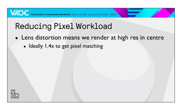
The lens distortion applied for viewing in the headset means we need to render at a high resolution in centre of the image Ideally this should be 1.4x1080p to get 1:1 pixel matching I'm going to show you a little video to explain
