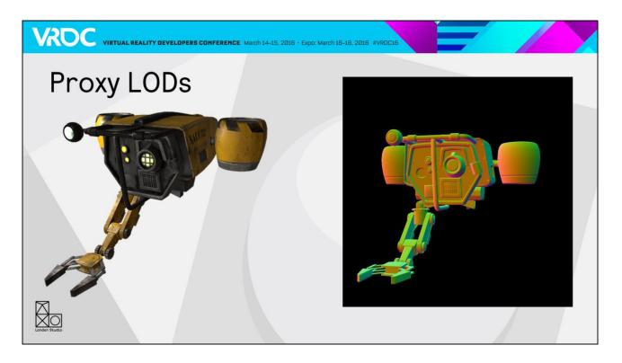
We run the model through Maya's automatic UV mapping to generate a new set of unique UVs, and use the vertex shader to flatten the model into UV space. Here's the process with world space normals.
