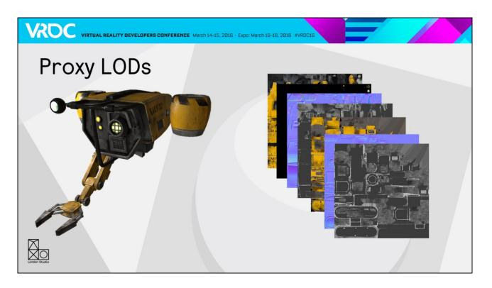
Here we have a drone from The Deep. It's a relatively simple shading setup, 2 materials and 7 textures. Obviously with layered shaders you can have a lot more inputs. The input mesh here is about 14k polys.
