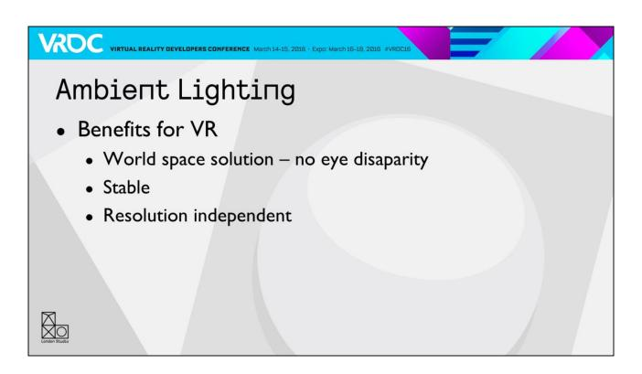
Lightfields is a good fit for VR. As well as the speed, it's a world space solution, so there's no difference between the eyes. It's stable, so there's no flicker or shimmering, and it's resolution independent, in that most of the work is done off screen.
