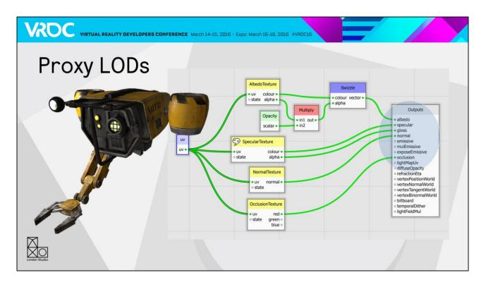
The first thing we do it to bake all the material outputs from the shader. These correspond with the values that we pass from our material editor into our lighting models. This is the shader that's used on the drone. As you can see, it's pretty simple, it doesn't really do much other than read a few textures and pass the values along.
