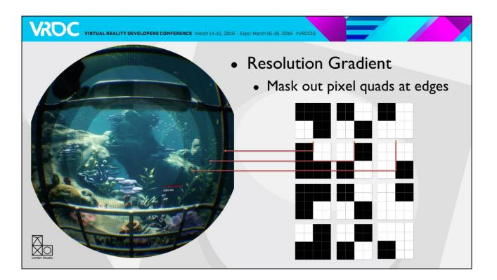
We mask out a dither pattern in increasing amounts, so 25%, 50% and then 75% of the pixels aren't rendered at the edges. We currently mask out 2x2 pixel quads, as masking out single pixels isn't GPU friendly, but I'll come on to this later.
