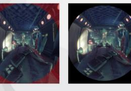
The left image shows what we render before distortion for the lenses. The red area isn't needed, so we mask it out. This saves us about 20% frame time for no visual loss. I think this is covered in all the VR SDKs at this point.
