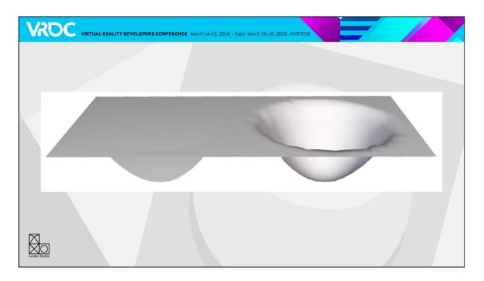
If you rotate joints, the normals work acceptably well – they just rotate with the joint based on the weighting. But facial animation largely uses translations rather than rotations, and that doesn't update the normal at all.
