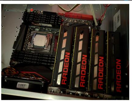
Precomputation Cruncher 4x AMD Radeon R9 Fury Nano
