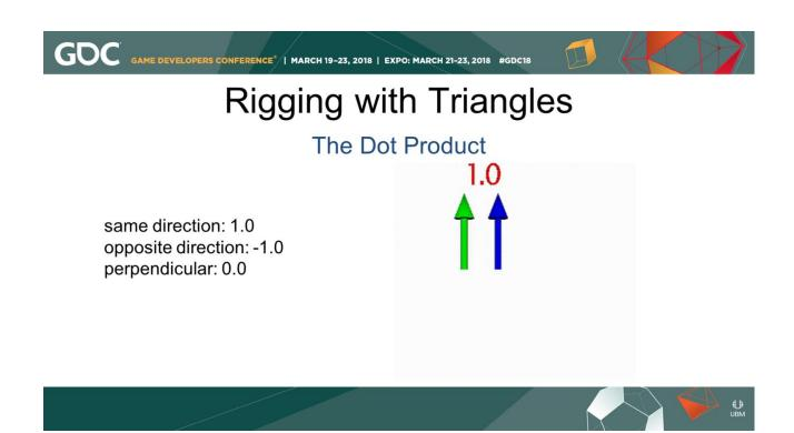
The dot product of two vectors pointing in the same direction is 1, pointing in opposite direction is -1, and two perpendicular vectors' dot product is zero. There are values in between as well: the dot product of vectors gives a similar result as the cosine of scalars.
