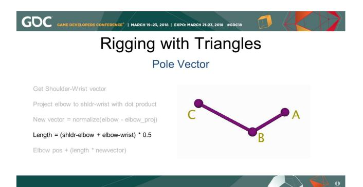
It's personal preference how far off the elbow we position the pole vector, but my rule of thumb is half of the length of the entire arm, or AB plus BC times 0.5.
