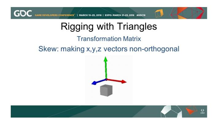
We can Skew the object by making x,y,z vectors non-orthogonal to each other.
