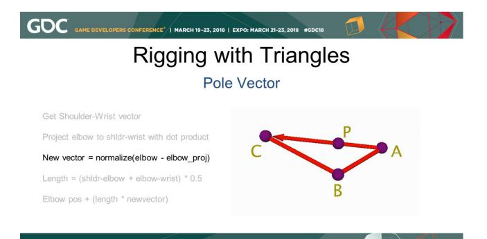
We make a new vector by subtracting the elbow position B minus P, and we normalize that vector.
