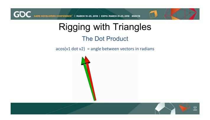
The ArcCosine of of the dot product of two normalized vectors is the ANGLE between the vectors in radians.
