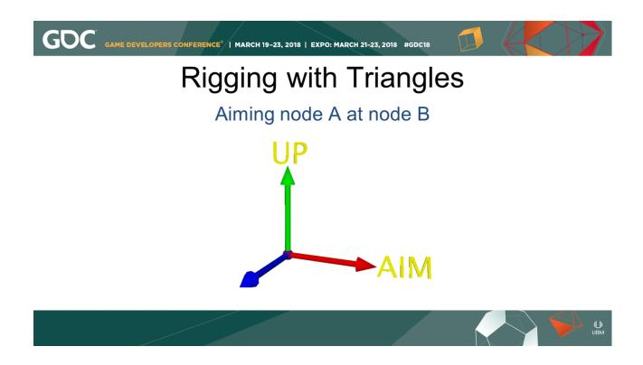
A's X axis will be the axis we aim at B, and its Y axis will be point as much toward C as possible.
