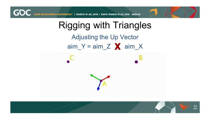
Now aim\_x and aim\_z are 90 degrees from each other, and aim\_Y and aim\_Z are 90 degrees from each other, aim\_x and aim\_y aren't necessarily 90 degrees from each other. So we get an adjusted aim\_Y by crossing aim\_Z and aim\_X.
