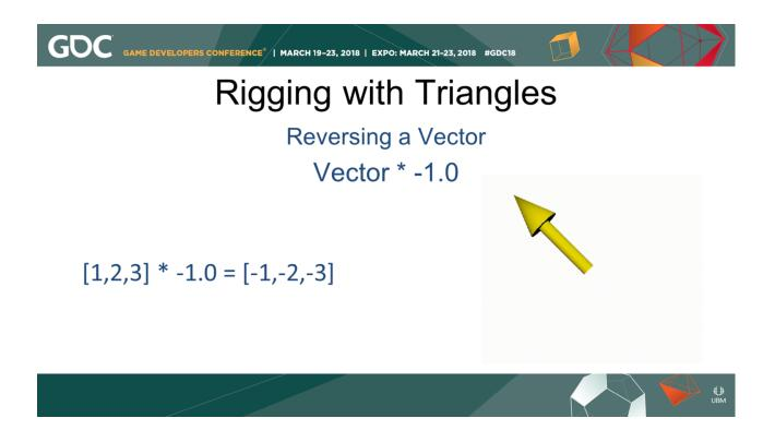
Reversing a vector is pretty easy: We multiply the vector by -1, which in turn just multiplies each element of the vector by -1, and the resulting vector points in the opposite direction.
