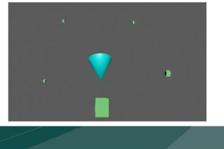
Here's a quick demo of a Pose Space node I wrote using the dot product to calculate a value indicating how much a driver object points toward a list of other objects. Remember, the dot product of two vectors pointing in the same direction is 1, so I'm just comparing one of the driver node's axes with the normalized vector of the target node's position minus the driver's position.
