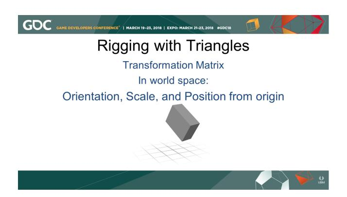
A Transformation Matrix In World Space describes an object's orientation, scale, and position from origin.
