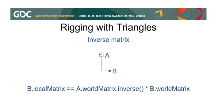
If B is the child of A, we can multiply the inverse of A's world matrix with B's world matrix to get the local transformation matrix of B. **()** UBM
