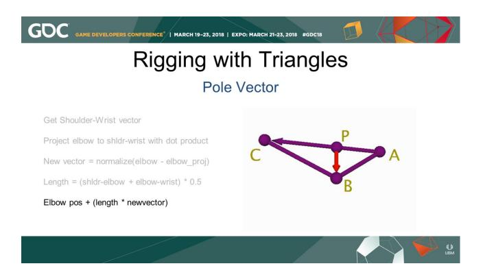
Finally, we set the position of the pole vector control: multiply the normalized PB vector times the length value we calculated, and add that to the elbow position B.
