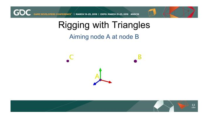
Here's some points in space, A,B, and C. A is currently aligned to the world, but we want to aim A at B, and use C as the upvector
