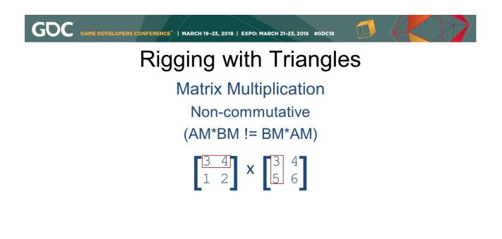
Matrix multiplication is non-commutative, in other words A times B doesn't necessarily equal B times A because the math involves multiplying the rows of the first matrix with the columns of the second. UBM
