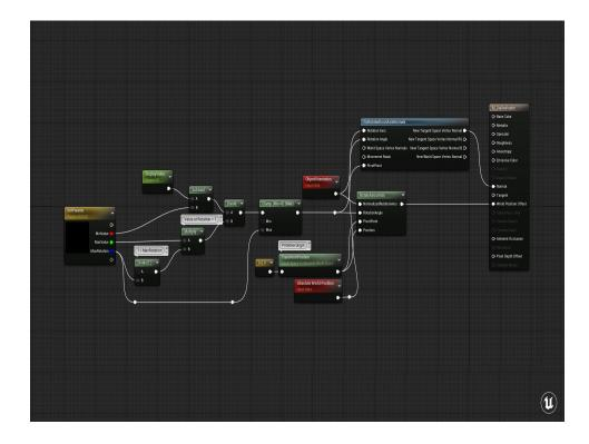
Luckily we've got a node that does that for you in Unreal already. We'll just hook up the required inputs, and pass the new output to the Normal input of the material node. Now our dial normals will be pointing in the correct direction based on how much their position has changed.
