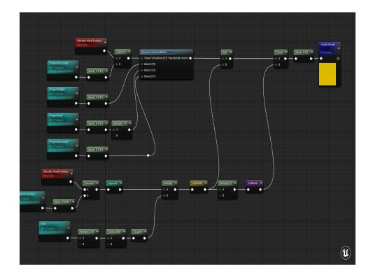
And because right now our "UVs" aren't centered at .5, .5 we need to bias it over by half the width of the texture and dividing that by the full width of the texture to get the values from 0 to 1.
