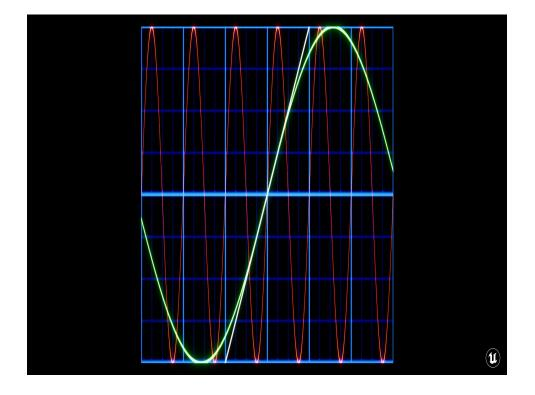
Then we need the tangent of our angle. The FOV is input as degrees, and in the Unreal Engine our material trig functions are in a period 1, or unitless. This is a big difference from your graphing calculator, which uses a period of 2pi. I graphed those out here so you can see the difference.
