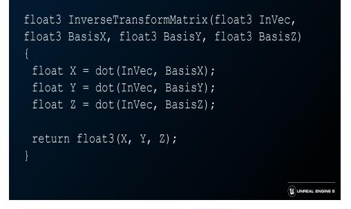
The InverseTransformMatrix material function, spelled out using functions available as graph nodes in the material editor.
