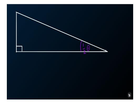
I know the FOV, and if a right triangle is half an isosceles triangle then I guess that means this angle is half the FOV
