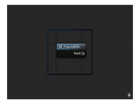
On the material side of things, I'm going to be putting all this logic into a Material Function to make it ever more portable. This is just going to output my UV values and I can use this any way I want in other materials.
