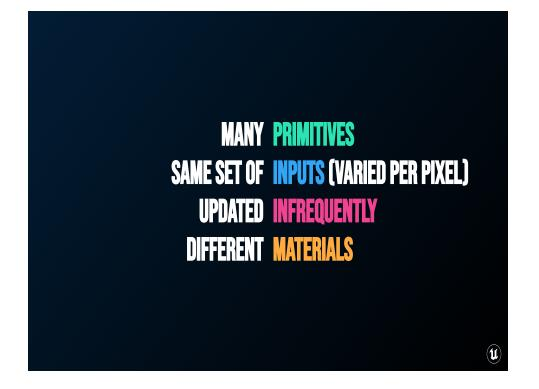
There's two sides to how we're going to use RVTs, but for the purposes of consistency on the *read* side of things, these are great for when you have many primitives that need to react to the same set of input data that varies per pixel, but that set of input data doesn't have to update every frame.
