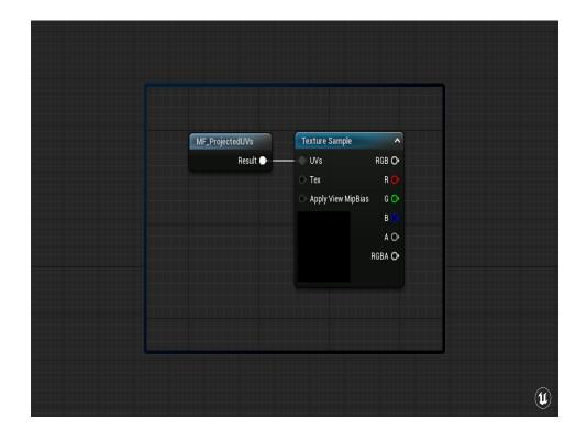
Then all you have to do is use that material function outputting its UVs into a texture sampler. For this example, this is all I need to look sample the looping video for the man behind the curtain. From here I can plug this into the rest of my emissive stack to blend it in however I need!
