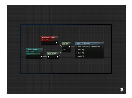
We just need to pass in the Vector to Transform, which is the WorldPosition-ProjectorLocation vector.
