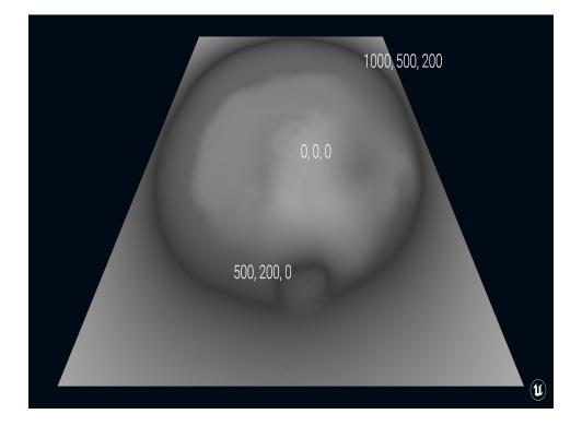
The great news is that one of the other channels to which you can write is *height*. This means there's a whole texture that's meant to associate a Z height value with a given X/Y Position. And if I write the height of the landscape out to that runtime virtual texture, then I can look up the height of the landscape at any point in the world in any material.
