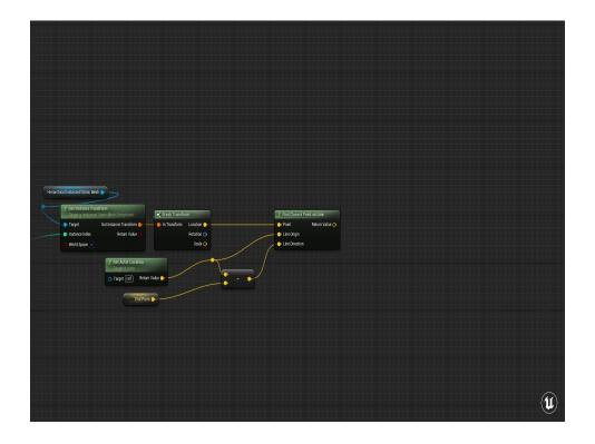
The line percent is a bit trickier, but luckily Unreal has a built in "get closest point along a line" node. For the point, I just ask the instanced component for the worldspace location of the instance we're operating upon. The origin of the line is the origin of the actor, and the direction is the Start -> End Vector.
