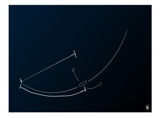
LinePercent is how far along the vector from Start to End is the chain placed, and the SwayAmount is a value we're going to calculate based on how far along the chain a given link is
