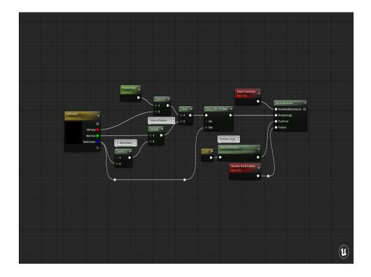
Now that we have a rotation value in the 0 to 1 range, we can use the RotateAboutAxis node to figure out how much we need to offset the position of each vertex.
