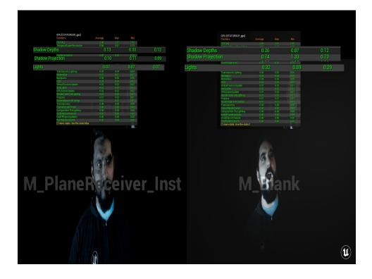
To test the performance differences here, I again set up a full-screen quad with two different materials: one that displays the projected texture like we were doing with the particles, and one that's just a default lit, grey material. When I swap to the grey material I switch to a three spot-light set that are each throwing Red, Green, and Blue light respectively, along with a light function material that's just playing the video.
