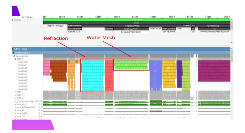
The water system first copies the scene color out to a secondary buffer and applies fog – this is for refraction. Then the water mesh renders to the full gbuffer like a regular opaque draw. Having an updated depth buffer has benefits for TAA in particular.
