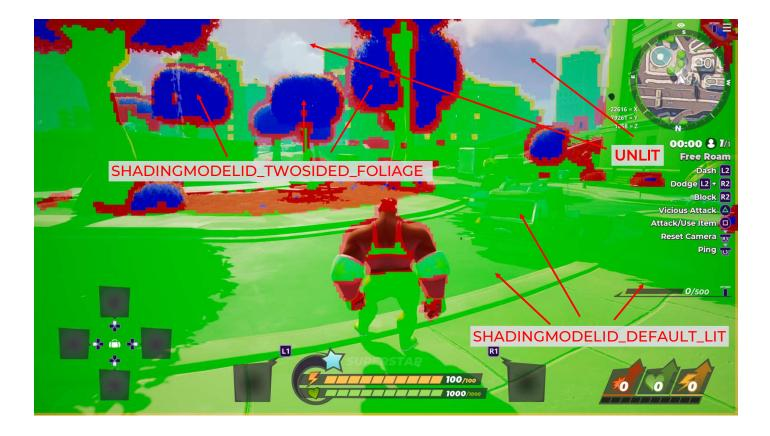
However, the most important thing this work took me to was the unlit tiles here, tiles that are culled entirely had the biggest impact on the running time. This got me thinking about how the tile classification could be used for culling workload from SSR + SSS as well, and that cost of running the classification would be shared across multiple steps of our rendering.
