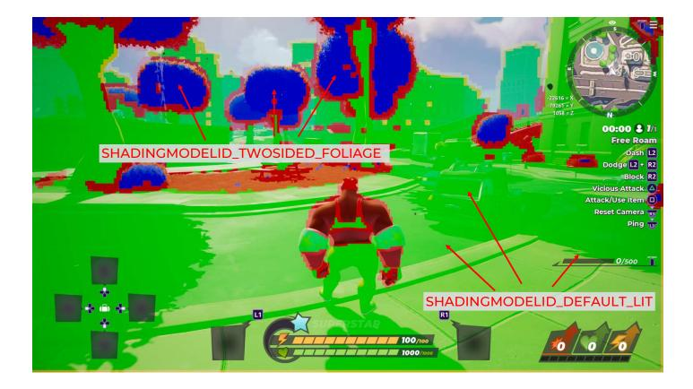
And here you can see a visualization of the tile classification in practice. The green tiles are default lit, the blue is all foliage, and the red contains a shading paths that are "complex" and run the full shader
