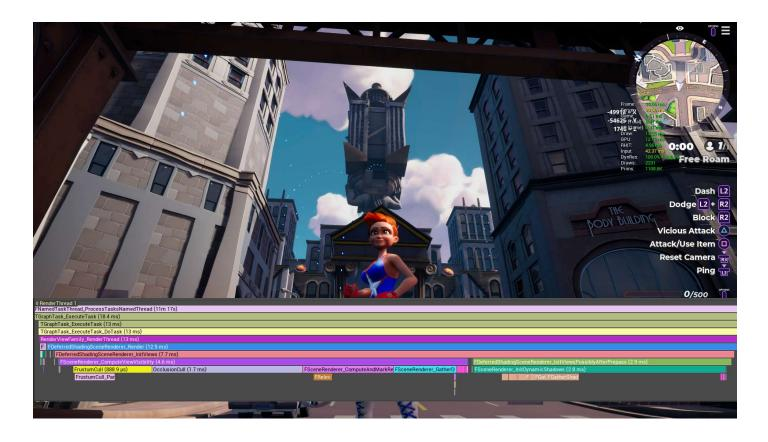
Here is an example of a challenging shot in front of some buildings that are made up of many primitives that are processed individually before instancing. You can see here that InitViews is taking up a hefty 7.7 ms, which is approaching half of our total frame time.
