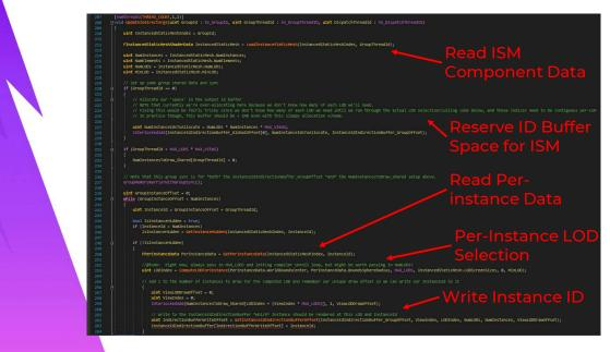
Let's take a look at that shader. Each ISM component gets a single group (the size of 1 wavefront) that allocates space into the ID buffer. This is done atomically as multiple groups are in flight at once. The some LDS is cleared to track the IndirectArgs and a barrier is inserted.
