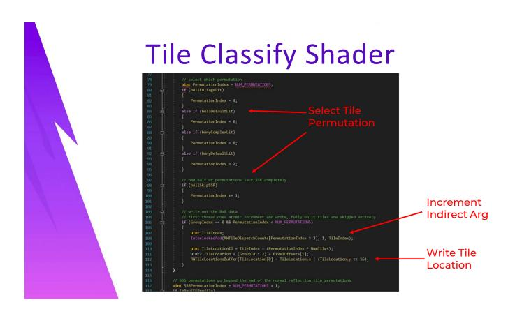
Then the shader permutation for the tile is selected based on the bits held in the MergedResult across the whole wave, and the result is written out by the first thread. An interlocked add occurs on the counts which gets a unique index for the tile that maps to the Tile Locations Buffer, which holds the pixel location for a given tile on the screen and will be used to reconstruct the pixel locations for each tile in the apply shaders.
