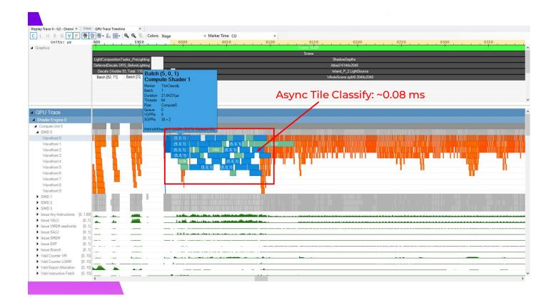
And we can actually do better, this classification job very nicely overlaps with shadow depth rendering using async compute, here you can see it overlapping with some vertex shading work before some pixel shader waves for masked materials run. This is frame dependent, but I generally see running it async save ~0.1 ms of frame time which makes the cost approximately 0.08 ms on a PS4.
