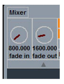
Fade in and Fade out timers. These allow the cross-fades between mixers to be tuned
